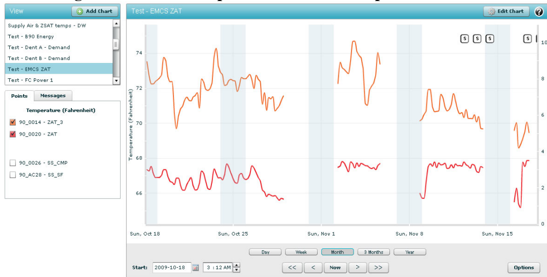
Figure 5. B90 Data Gaps from Zone Air Temperature Sensors
